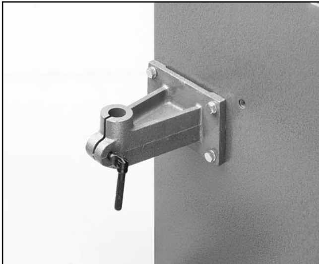
Figure 4. Lead screw bracket Installed.
